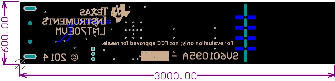
Figure 6-6. Bottom Assembly Layer
