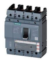
circuit breaker 3VA5 UL frame 250 breaking capacity class C 100kA @ 480V 4-pole, line protection TM210, FTFM, In=100A overload protection Ir=100A fixed short-circuit protection Ii=10 x In N conductor protection 100% without connection
