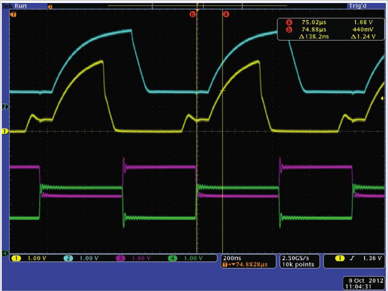
Figure 11. Differential bus waveform
