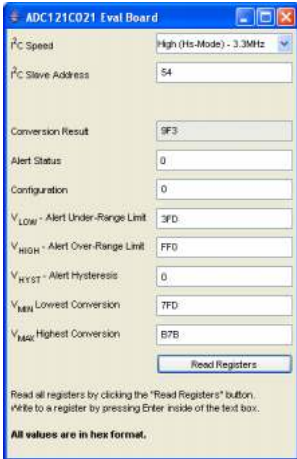
Figure 10: ADC121C021 Control Panel
