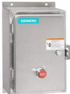
Non-reversing motor starter Size 2 1/2 Three phase full voltage Solid-state overload relay OLRelay amp range 25-100A 240VAC 50HZ / 277VAC 60HZ coil Combination type Water/dust tight non-corrosive
