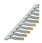
Crimp contact, Socket, rolled, Taped articles, number of pieces per reel: 500, contact diameter: 1 mm, crimp range: 0.22 mm<sup>2</sup> ... 0.56 mm<sup>2</sup>, Item is lead-free in accordance with RoHS II without Exemption 6c (Pb <0.1%)
