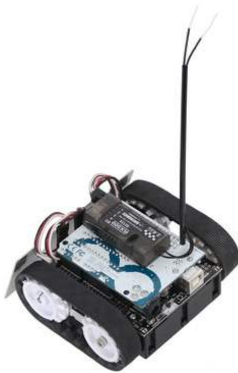
A Zumo robot with an RC receiver attached to make a radio-controlled vehicle.
