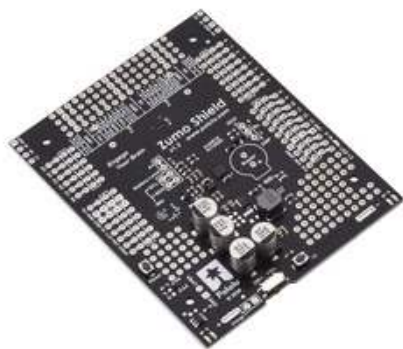
Zumo Shield for Arduino, v1.3, as it ships (assembled with surface-mount components only).
