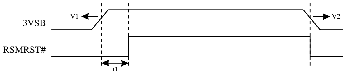
Figure 14-5 Mechanism of Resume Reset Logic
