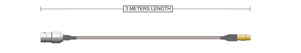
Connector A 112631 BNC Jack Straight Brass Nickel + Heatshrink 50 Ohm RG-178 Continuity/Hi-Pot Connector B 262117 MMCX Jack Straight Brass Gold + Heatshrink
