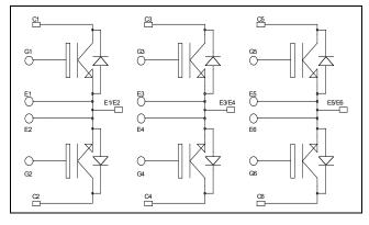
$V_{CES} = 600V$  $I_{C} = 100A$  @  $T_{C} = 80^{\circ}C$
