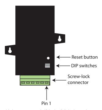
The adapter is switch-selectable between RS-422 half duplex/full duplex, and RS-485 modes (see DIP switches on page 24). The function for several pins varies between RS-422 and RS-485 modes.
