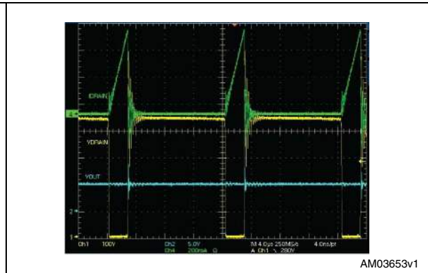
Figure 12. Drain current and voltage at peak load 265 V AC
