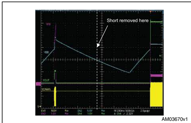
Figure 30. OLP: steady-state, short removal and restart
