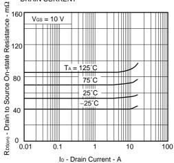
DRAIN TO SOURCE ON-STATE RESISTANCE vs.
