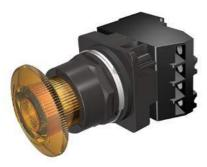
30mm BlackMax, Epoxy Coated Corrosion Resistant Complete Metal Unit Illuminated Twist-to-Release Full Voltage, 120V AC/DC LED Lamp Mushroom Head Cap Small 1.79" (45 mm) Plastic Cap, Amber 2 Position Maintained, Twist-to-Release with 1 N.O. - 1 N.C. Heavy Duty Contacts, A600/P600 UL Listed, CSA Certified NEMA 1,3,3R,4,4X,12,13 & Automotive Standards
