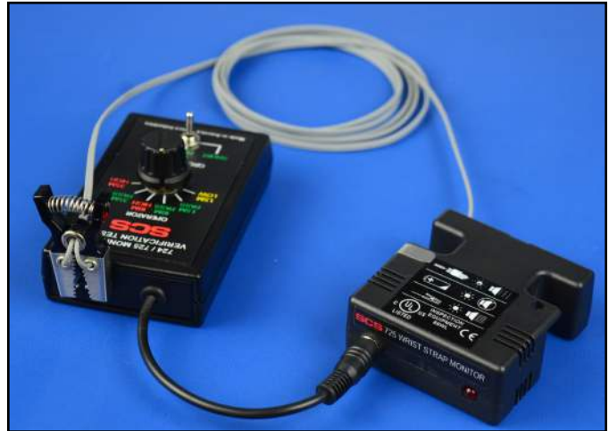
Figure 4. Using the Verification Tester with the 725 Portable Wrist Strap Monitor
