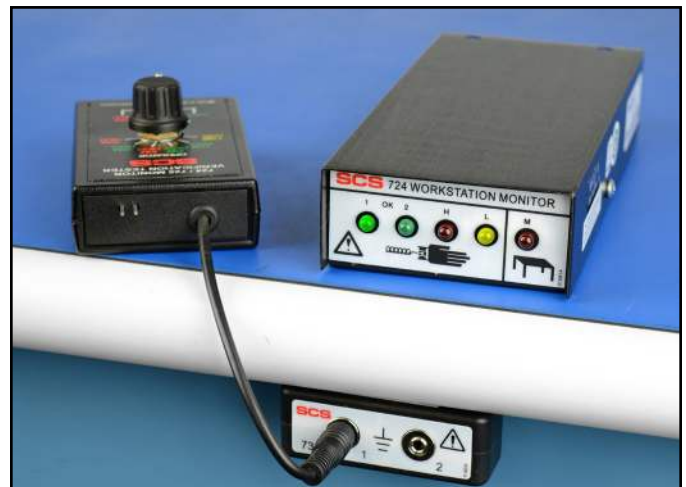
Figure 3. Using the Verification Tester with the 724 Workstation Monitor
