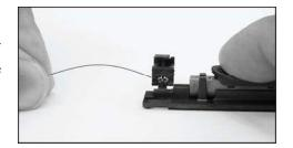
Release the bow in the fiber and fully close the left buffer clamp. Again, you will hear an audible snap.
