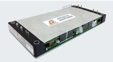
The AGF800 series of isolated DC-DC converters is designed for RF applications such as high power wireless base stations that use both 28V for LDMos and 48V for gallium nitride (GaN) technology for increased power density and efficiency
