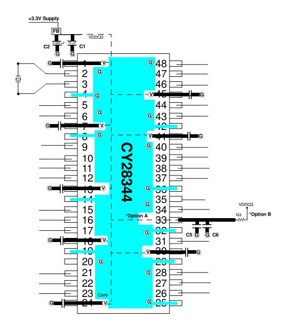
FB = Dale ILB1206 - 300 or 2TDKACB2012L - 120 or 2 Murata BLM21B601S Ceramic Caps C1 = 10 - 22  $\mu F$  C2 = 0.005  $\mu F$  C5 = 0.1  $\mu F$  C6 = 10  $\mu F$  = VIA to GND plane layer = VIA to respective supply plane layer Note. Each supply plane or strip should have a ferrite bead and capacitors.
