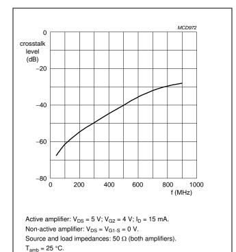
Fig.19 Crosstalk as a function of frequency: Output level of non-active amplifier related to output level of active amplifier; typical values.
