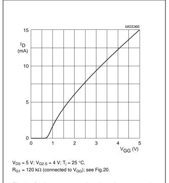
Fig.8 Drain current as a function of gate 1 supply voltage (=  $V_{GG}$ ); typical values.
