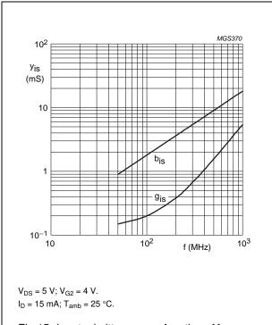
Fig.15 Input admittance as a function of frequency; typical values.
