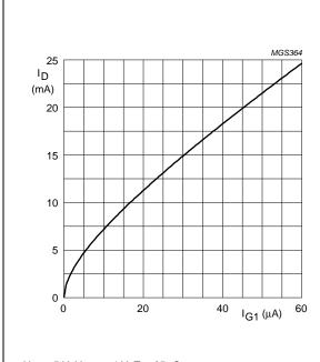
$V_{DS}$  = 5 V;  $V_{G2\text{-}S}$  = 4 V;  $T_{j}$  = 25 °C.
