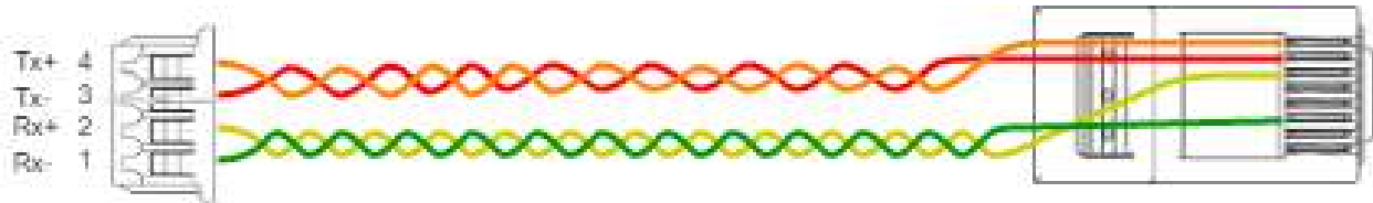
Figure 6: Ethernet cable pinout
