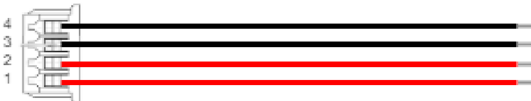
Figure 4: Voltage input cable pinout (red = V+, black = GND)
