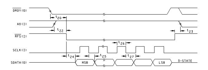
External-clocking mode, output data read operation
