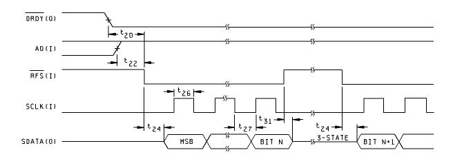
External-clocking mode, output data read operation (&&S returns high during read operation)
