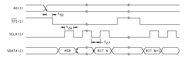
External-clocking mode, control/calibration register write operation ( & returns high during write operation)
