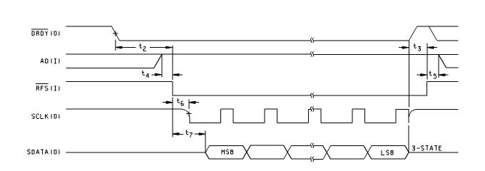
Self-clocking mode, output data read operation
