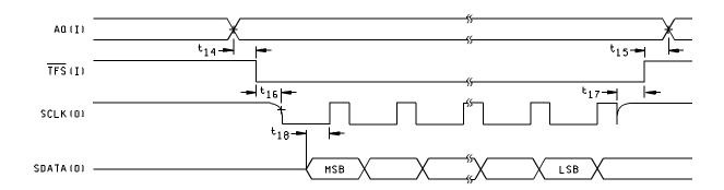
Self-clocking mode, control/calibration register write operation
