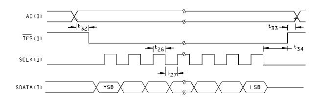
External-clocking mode, control/calibration register write operation
