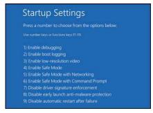
That is all there is to it. Your PC will then reboot and you will be able to install unsigned drivers without any error message. After the driver has been correctly installed an orange logo should appear in the device manager when the USB dongle is plugged into the PC:
