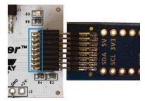
The pinning of the connector is mirrored on the SensorXplorer board, so there is an option of connecting the board the other way around; however, this is not recommended, as the connector has pins on the SensorXplorer board side of the connector, as indicated above. If the sensor board is connected the other way around, care must be taken not to push the sensor board all the way through, as this will lead to a short circuit.
