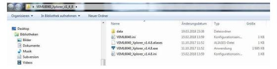
The data folder contains the required DLLs for the executable to run and for the hardware communication to function. This folder should not be moved or deleted, as the executable references it as a relative path.
