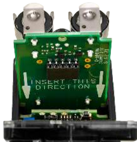
Figure 1. Q45 battery board
