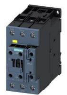
power contactor, AC-3e/AC-3, 41 A, 18.5 kW / 400 V, 3-pole, 83-150 V AC/DC, 50/60 Hz, with integrated varistor, auxiliary contacts: 1 NC, screw terminal, size: S2, F-PLC-IN
