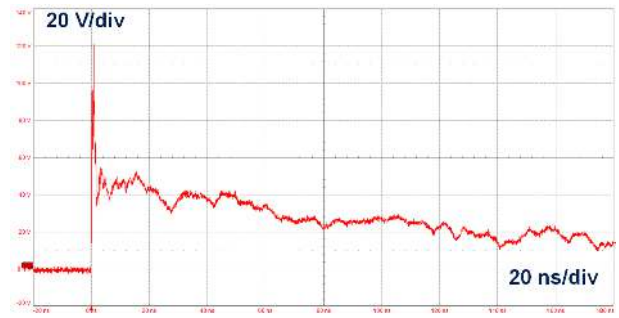
Figure 9. Response to ISO 10605 - C = 150 pF, R = 330 \Omega (+8 kV contact )
