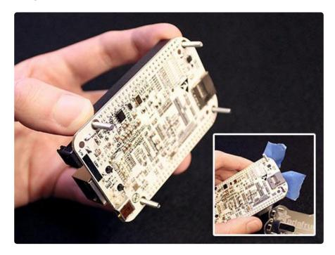
Slide a nylon spacer over each of the four screws. VERY IMPORTANT: Use ONLY the spacers included with the kit. DO NOT use wider standoffs or spacers in their place, and SUPER ESPECIALLY DO NOT use hex-nuts as a makeshift standoff/spacer. The component clearances on the BeagleBone are very close, and using the wrong spacers could result in components being crushed!
