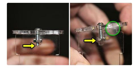
Insert the BeagleBone base plate into the case by inserting the alignment studs into the back face, then pivot the board into place and press the front face flush.
