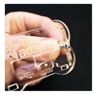
Install the second side piece using the same technique, then repeat with the opposite end face plate, making sure the "up" orientation is the same. It's okay if the box isn't perfectly square at this stage.
