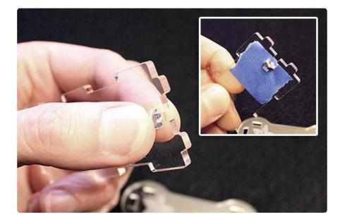
Position one of the end pieces over the alignment studs, then insert a screw through the corresponding hole for the nut. Tighten with gentle finger pressure for now.
