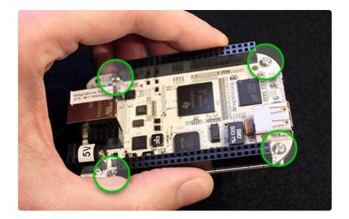
Flip the board over, using fingers and thumb to hold the screws in place. If this is a dexterity challenge, the screws can also be held with tape:
