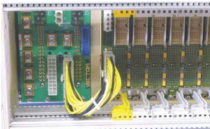
4626 ATX connection to cPCI backplane or screw terminals (power bug) wiring
