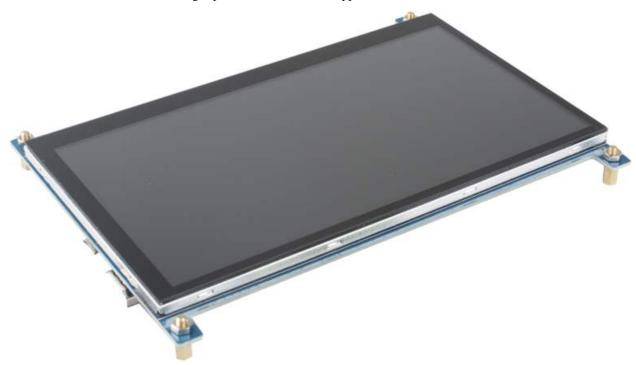
Take out M3 nuts and M3x8+6 single-pass brass standoff to support the 7-inch touch screen.
