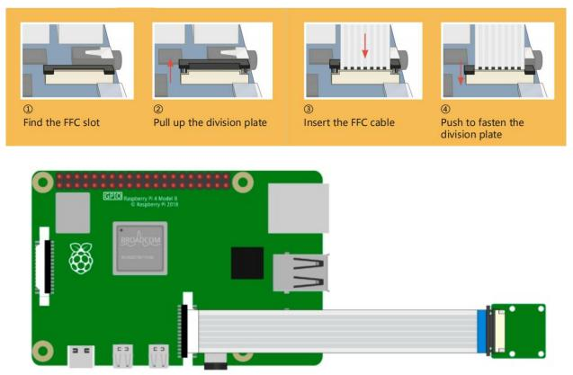
Warning: Do not install the camera with the power on, it may damage your camera.
