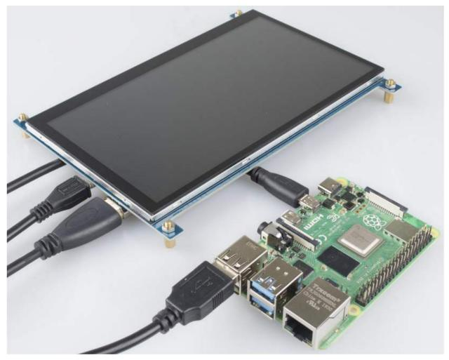
Plug the USB power supply into a socket and connect it to your Raspberry Pi's power port, and you may find a red LED lighting up on the Raspberry Pi, which indicates that Raspberry Pi is connected to power. As Raspberry Pi starts up (also called booting), raspberries appears in the top left-hand corner on your screen. After a few seconds, the Raspberry Pi Desktop will appear.
