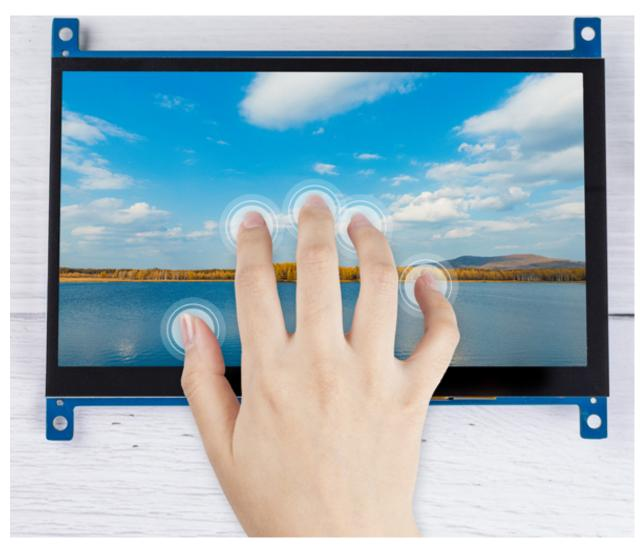
7-inch touch screen supports Raspbian/Win7/Win8/Win10(Plug and play), Android/Linux (need to be configured first). Equipped with Micro USB and HDMI port support, the screen can be connected to the device via HDMI interface and be powered via USB. Achieving touch function powered by USB doesn't need power cord or drive-free.
