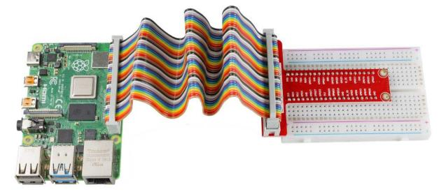
Connect the 40 pins of the Raspberry Pi to a breadboard according to the diagram below.
