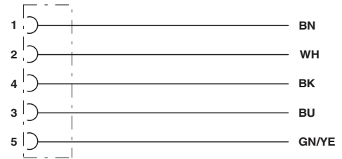
Contact assignment of the M12 sockets
