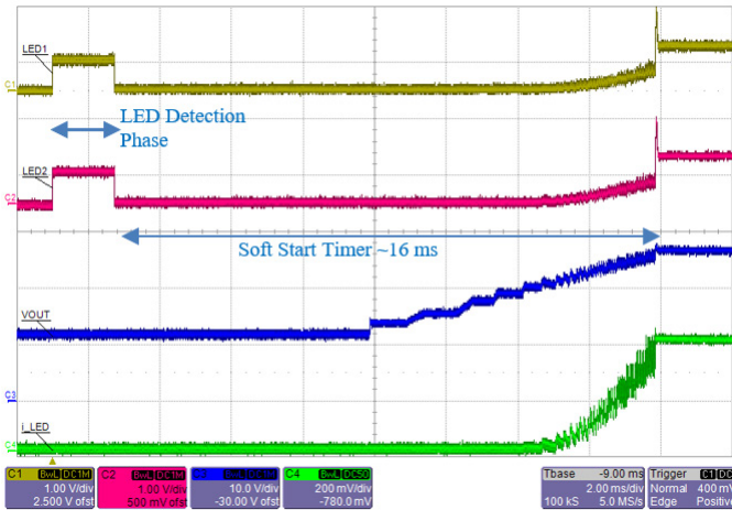
Figure 7: A80603-1 normal startup showing all channels passed LED Detection phase. Note longer soft start timer.
