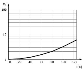
Formula:  $\pi_t = \exp(1,8.(t/tm)^2)$ with: t = using temperaturetm = maximum temperatureCurve for  $tm = 125^{\circ}\text{C}$
