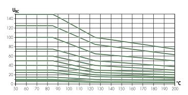
The category voltage ( $U_c$ ) is consequently the maximum DC voltage which can be applied continuously at +125°C.
