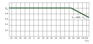
For the types which can be used up to 200°C, the voltage must be derated between +85°C and +200°C according to the following curve.
