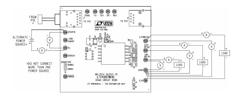
Figure 1. Proper Measurement Equipment Setup
