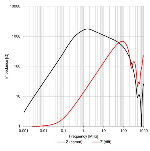
CHECKED REVISION DATE (YYYY-MM-DD) GENERAL TOLERANCE PROJECTION METHOD HasA 004.001 2021-01-08 DIN ISO 2768-1m **WE-CMB HC Common Mode** Würth Elektronik eiSos GmbH & Co. KG **Power Line Choke** ORDER CODE EMC & Inductive Solutions WURTH ELEKTRONIK Max-Eyth-Str. 1 7448227005 74638 Waldenburg MORE THAN YOU EXPECT SIZE/TYPE STATUS Tel. +49 (0) 79 42 945 - 0 BUSINESS UNIT PAGE www.we-online.com Valid 2/6 Type S eiSos eiSos@we-online.com
