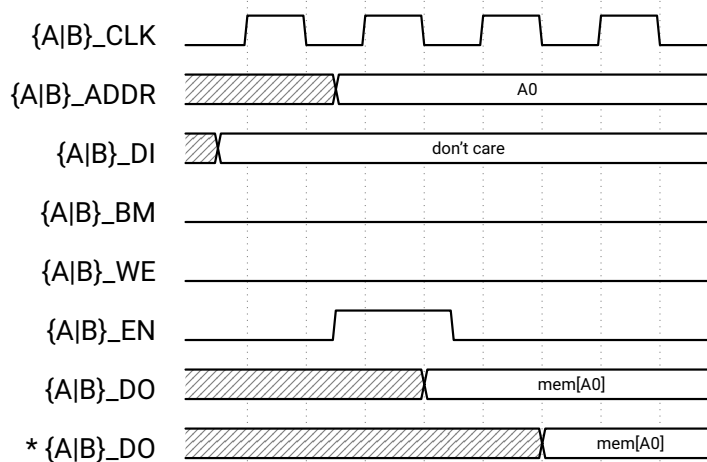
Figure 2.14: Timing diagram of a single read access with optional (*) output register
