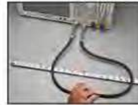
** Phase stability data IAW Times' phase/flex test criteria as demonstrated above. A brand new cable can have a break-in period of several hundred flexes.
