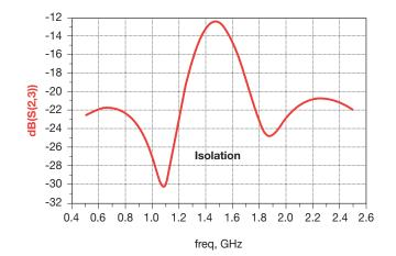
Note: Measurements were taken using an Anritsu 4 port VNA; Diplexer was mounted on a custom evaluation board. To reduce systematic errors from the VNA, the coaxial measurement cables, and evaluation board, a Short-Open-Load-Thru (SOLT) calibration was performed, using a custom fabricated calibration substrate. This is the most common coaxial calibration methods.
