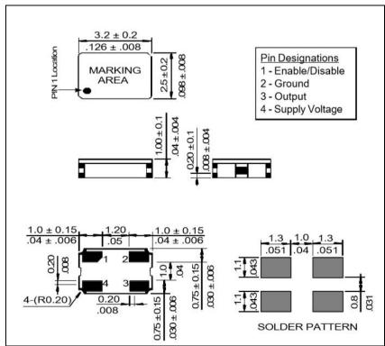
NOTE: A capacitor of 0.01 µF between Vcc and Ground is recommended
