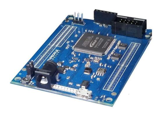
The MaxProLogic is an FPGA development board that is designed to be user friendly and a great introduction into digital design for anyone.
