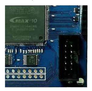
This connector uses the standard Altera Blaster connector pinout.
