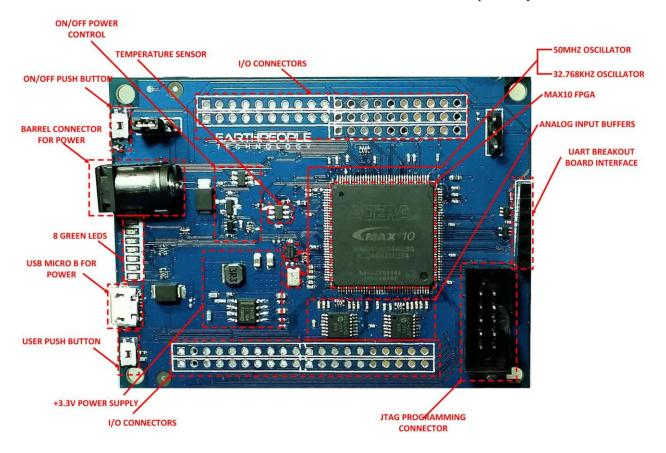
Figure 2 EPT-4CE6-AF Block Diagram
