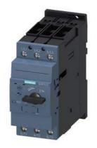
Circuit breaker size S2 for motor protection, CLASS 10 A-release 9.5...14 A N-release 208 A screw terminal Standard switching capacity
