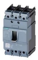
circuit breaker 3VA5 UL frame 125 breaking capacity class S 25kA @ 480 V 3-pole, line protection TM210, FTFM, In=25A overload protection Ir=25A fixed short-circuit protection Ii=12 x In UL489 SB (naval), 50 deg. cel. cable connection on both sides
