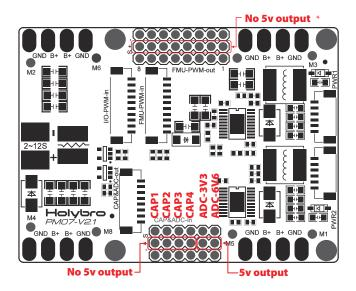
\*Note: If using a plane or rover, the 8 pins power rails of **FMU PWM-OUT** along with a BEC equipped ESC or a standalone 5V BEC or a 2S LiPo battery must be used to supply power to servos. Be careful with the voltage of servo you are going to use here.
