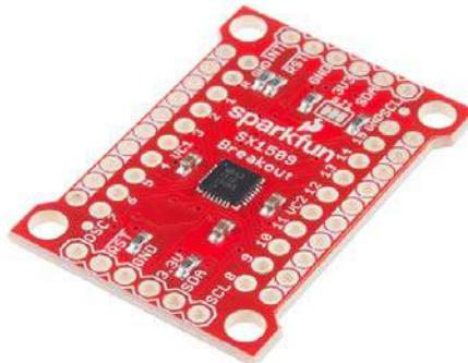
The SX1509 is a **16-channel** GPIO expander with an **I<sup>2</sup>C interface** – that means with just two wires, your microcontroller can interface with 16 fully configurable digital input/output pins.
