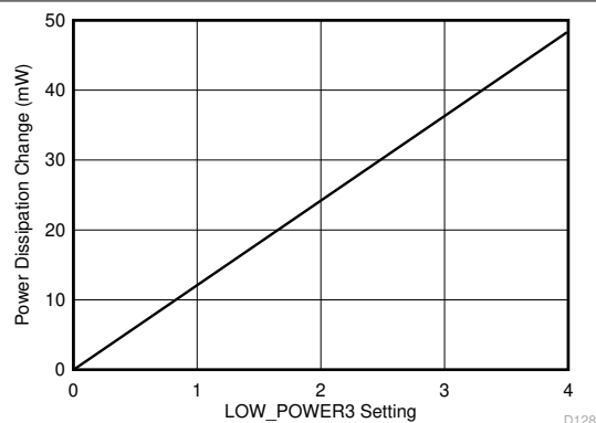
Figure 8-11. Power Dissipation Change vs LOW_POWER3 register setting
