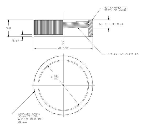
Start threads first or last depending on the panel thickness. Thick panels -1/8" -1/4" – Threads first.
