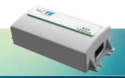
The NEVALO 25W triac dimmable LED driver is a high efficiency, power factor corrected supply with a unique color coded, keyed interconnect design that ensures optimal power is delivered to LEDs. The driver is designed with built-in voltage and thermal protection and is warranted for 5 years when used with the NEVALO SSL System.
