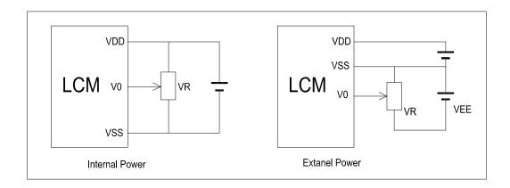
$V_{DD^{\sim}}V_0$ : LCD Driving voltage
