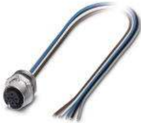
Sensor/actuator flush-type socket, 5-pos., M12 SPEEDCON, A-coded, front/screw mounting with M16 thread, with 1 m TPE litz wire, 5 x 0.34 mm<sup>2</sup>
