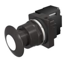
30mm BlackMax, Epoxy Coated Corrosion Resistant Complete Metal Unit Illuminated Push-Pull Operator Full Voltage, 120V AC/DC Incandescent Lamp Mushroom Head Cap Small 1 3/4" (44.5 mm) Metal, Black with White Lens 3 Position Momentary UL Listed, CSA Certified NEMA 1,3,3R,4,4X,12,13 & Automotive Standards
