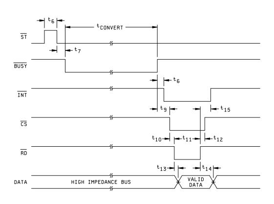
FIGURE 8. ADC mode 1 interface timing waveforms.
