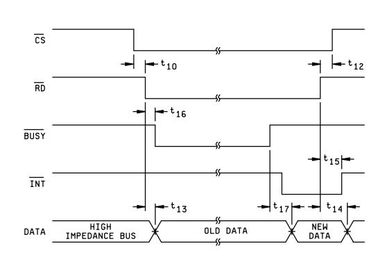
FIGURE 9. ADC mode 2 interface timing waveforms.
