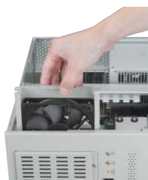
Easy-to-maintain cooling fan
